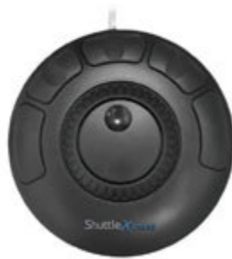
Figure 1: The Contour Design Shuttle Xpress jog & shuttle wheel used in our experiments
